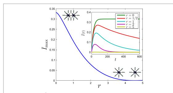
**Figure 2.** Maximum value of  $\bar{I}$  as a function of the distance r for two two-level atoms radiating in the electromagnetic vacuum. As expected, the amount of correlations in the dynamics decreases with r. In the inset,  $\bar{I}$  is represented as a function of time for different distances r between atoms ( $\omega = |\boldsymbol{d}|/2 = 1$ ,  $\theta = 0$ , see appendix  $\mathbb{C}$ ).
