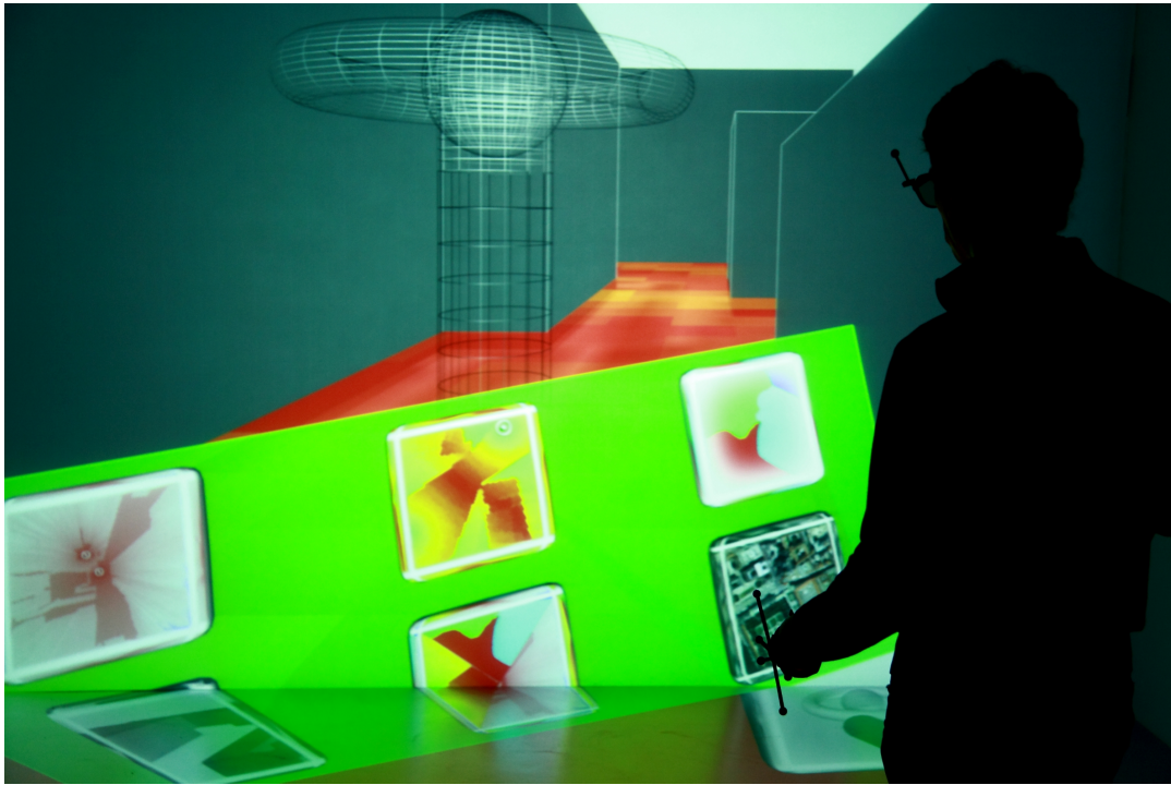
Figure 2.20.: User stands in the VE with a tracked marker attached to his non-dominant hand and a tracked pointing device in his dominant hand. His left hand is slightly raised to look at a panel for system control. The selection of the panel icon is done with the pointing device in his right hand. Upon completion the panel is hidden by lowering the non-dominant hand.
