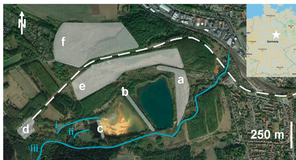
Figure 2. Schematic illustration of the TSF Bollrich's near environment: (a) marks the main dam, (b) the middle dam, (c) the water retention dam, (d) the disused processing plant, (e) a glider airfield, and (f) the disused landfill Paradiesgrund. The neutralisation sludge between the dams (b, c) is yellowish. The white dotted line marks the disused railway connection from Oker to the processing plant, (i) the stream of neutralised mine water, (ii) the connection between the pond Gelmketeich and the water retention pond, and (iii) the river Gelme. Adapted after Google Earth [50].
