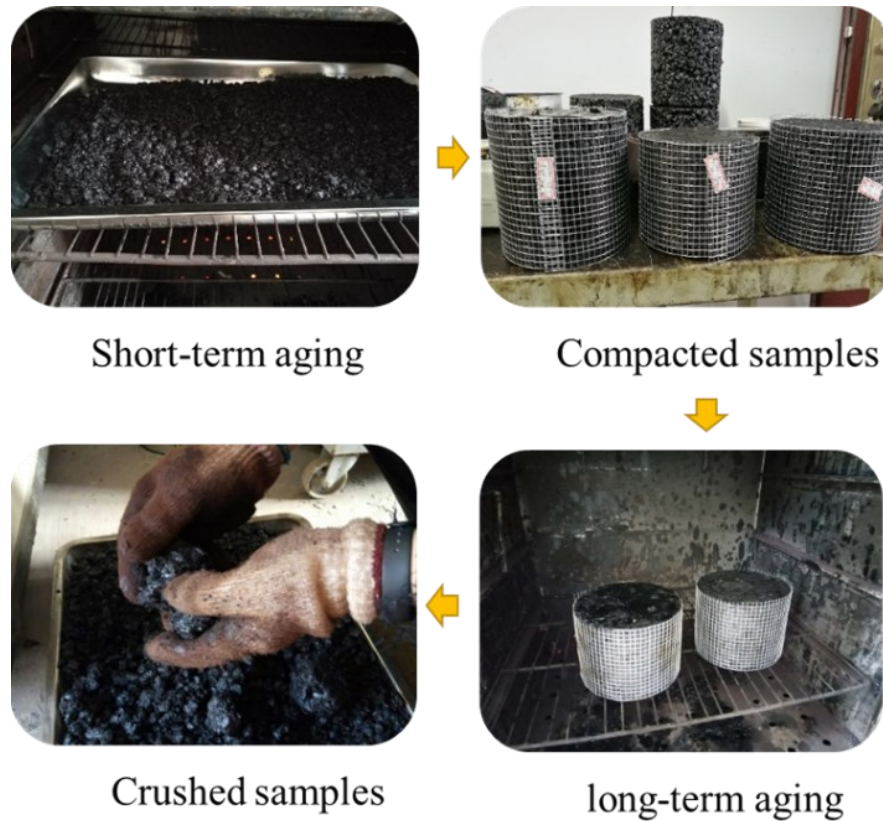
Figure 2.4 The process illustrating RAP production
