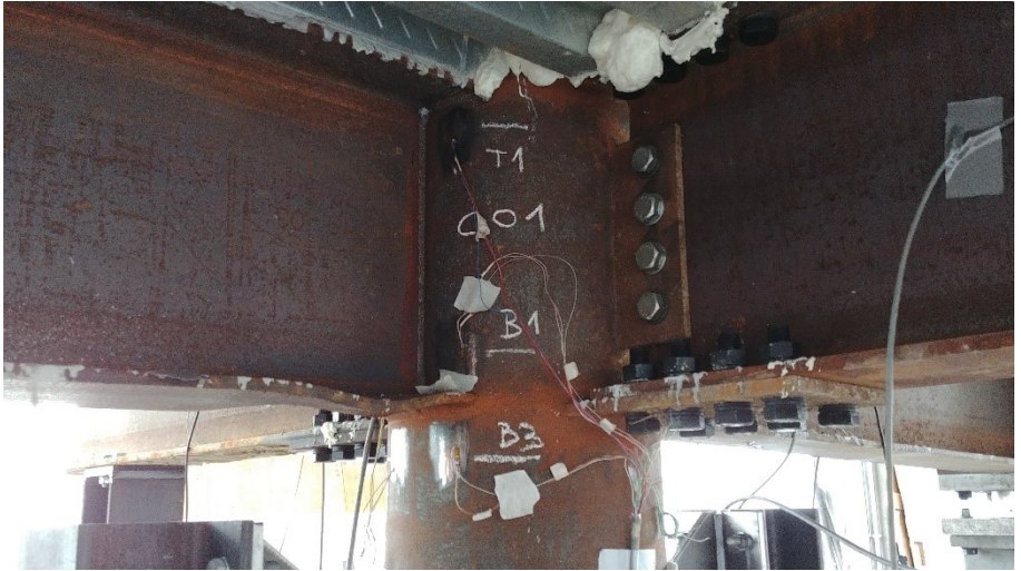
Figure 8.22 Local buckling of the lower compressed flange of the passing-through beam in the main direction of specimen C7
