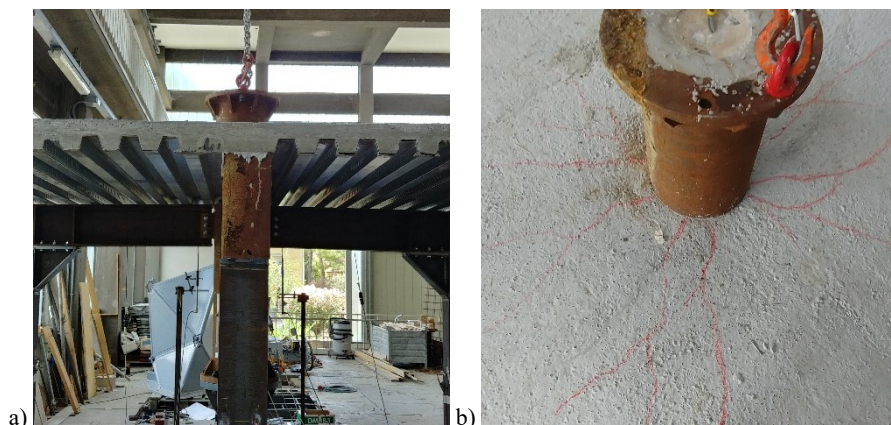
Figure 8.15 Failure modes exhibited in the monotonic test of the four-way specimen C5: a) rotation of the external girders due to the sliding of the bolted connections, b) cracking of the slab in the tension
