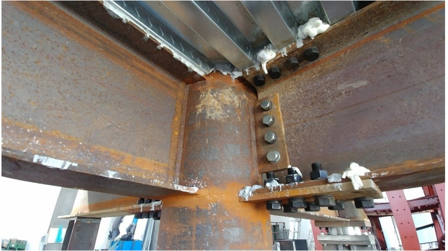
Figure 8.19 Four-way specimen C7 tested under vertical loads
