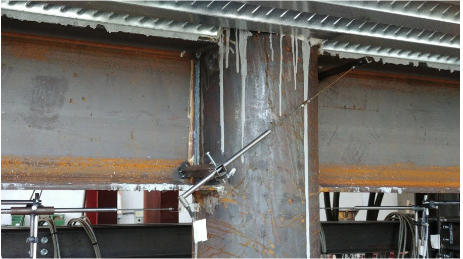
Figure 9.14 Two-way specimen C3 with the passing-through continuous beam
