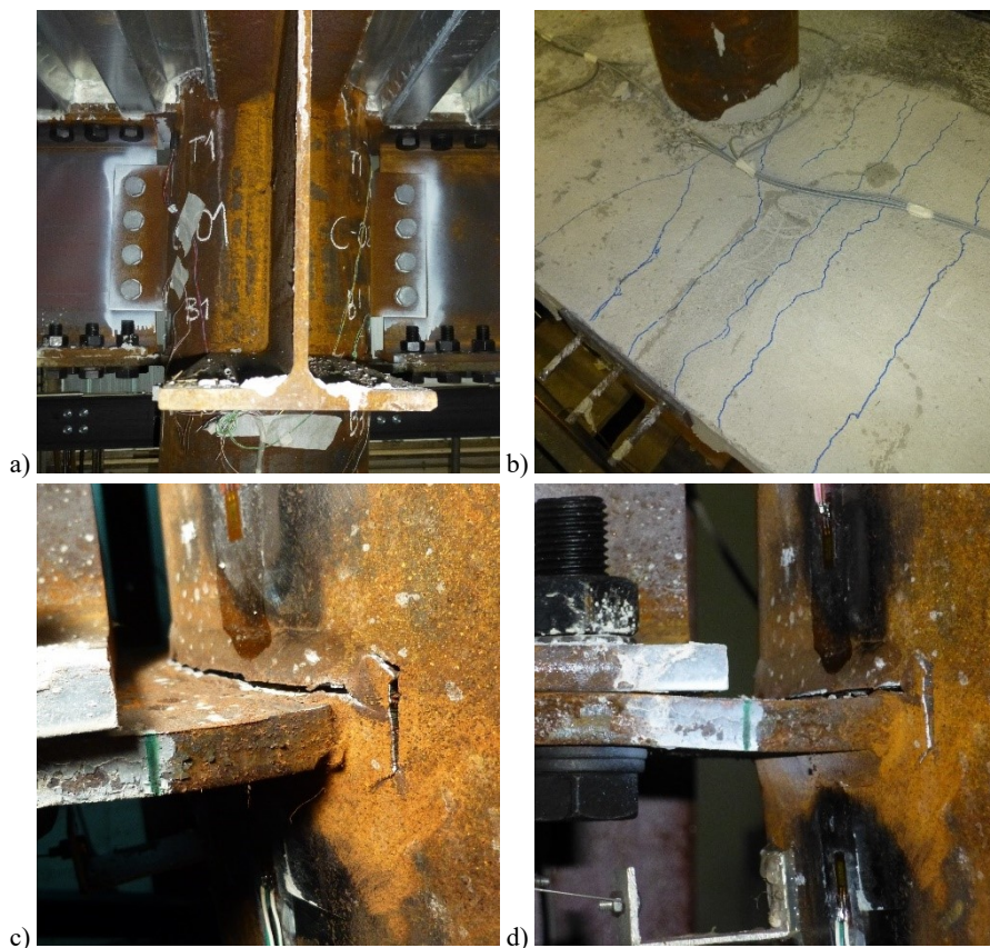
Figure 9.35 Failure modes exhibited in the test of the four-way specimen C7-2: a) sliding of the bolted connection of the flanges and web external girders, b) cracking of the concrete slab in tension, c) tearing of the welds around the bottom plate in tension, and d) opening of the gap due to the tension force applied by the column wall in tension
