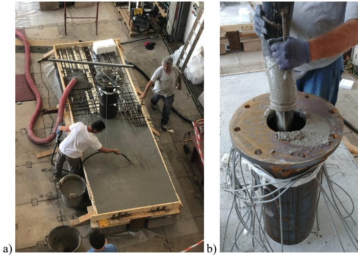
Figure 7.31 Fabrication of composite specimens: a) casting of the concrete slab, and b) filling of the tubular steel column
