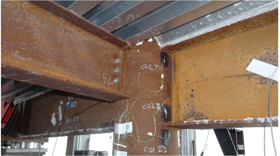
Figure 8.16 Four-way specimen C6 tested under vertical loads
