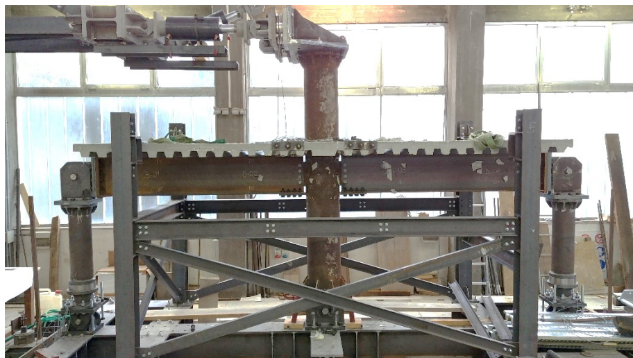
Figure 9.13 Horizontal loading test setup for composite specimens (University of Pisa)
