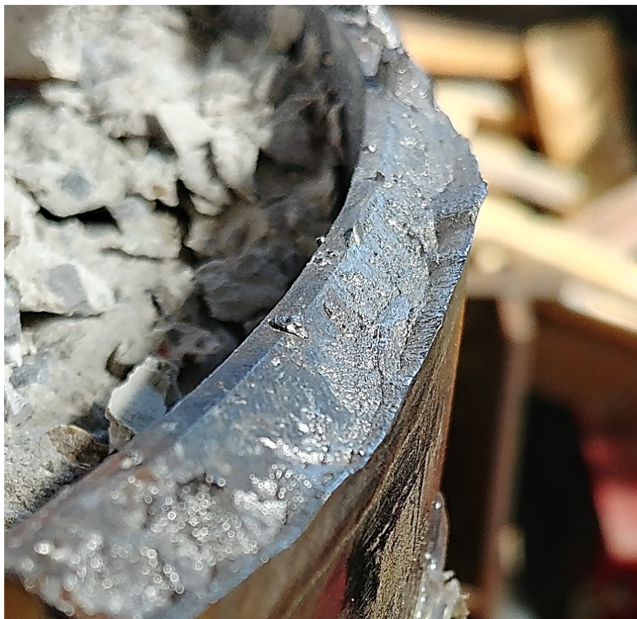
Figure 9.36 Region of lesion formation in the welds; it is possible to notice that, in the welding process, the base material did not melt on the laser cutting-worked surface
