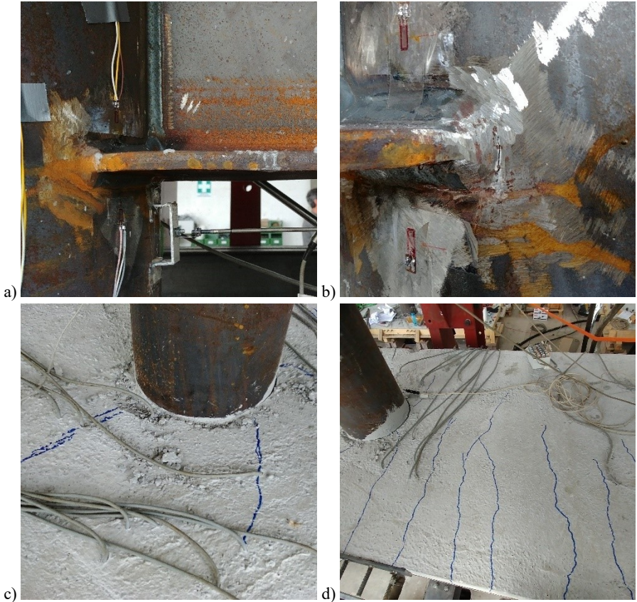
Figure 9.17 Failure modes exhibited in the monotonic test of the two-way C3 specimen: a) local buckling of the compressed lower beam flange, b) cracks in the welds in the tension region, c) crushing and lesions in the compressed concrete slab, and d) lesions in the tensioned slab
