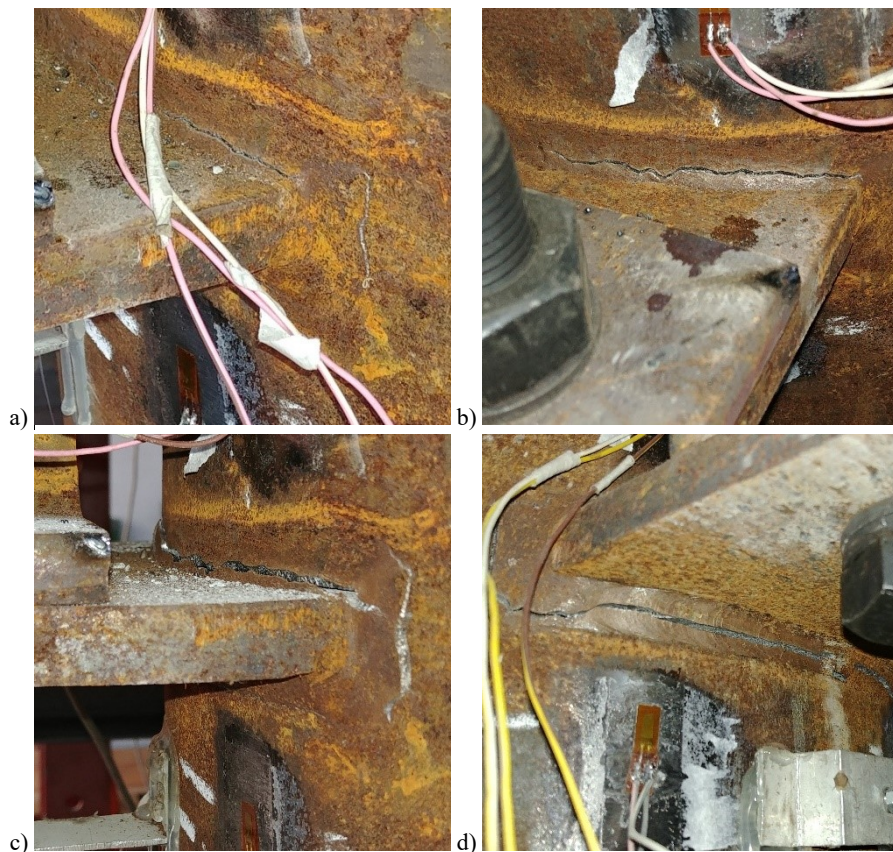
Figure 9.28 Failures of the penetration welds: a) first lesion exhibited in the first cycle at 60 mm, b) propagation of the lesion to the column wall in the first cycle at 80 mm, and c) in the cycles at 100 mm, and d) welds in the end of the test
