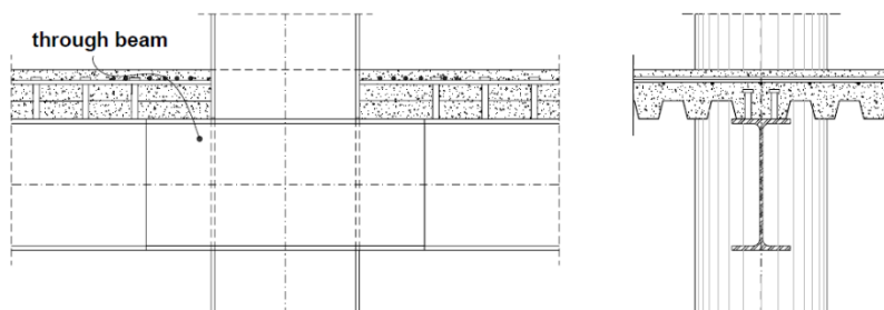
Figure 2.12 Connection made by a passing-through beam portion (Alderighi 2007)
