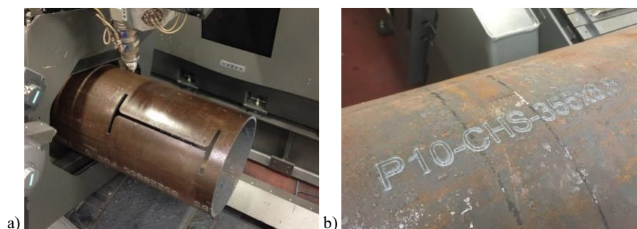
Figure 5.7 Laser cutting operations on column: a) slots realization on CHS-column, and b) part identification made by the laser cutting machine (Castiglioni et al. 2016)
