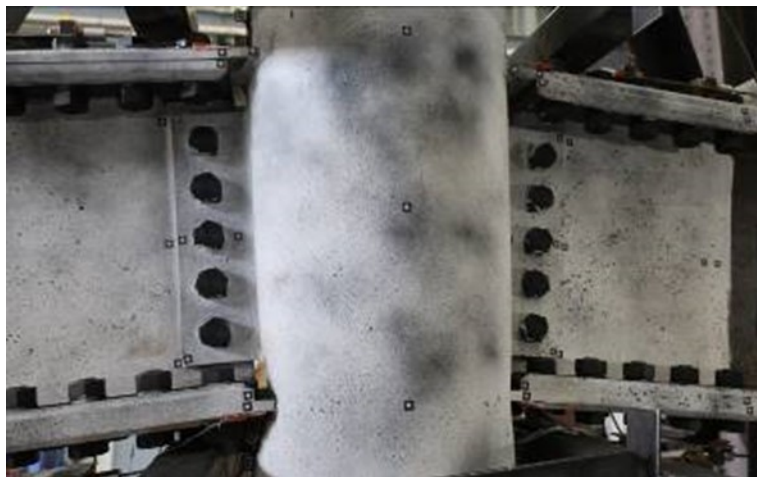
Figure 6.18 Specimen C4-4B-1 at failure
