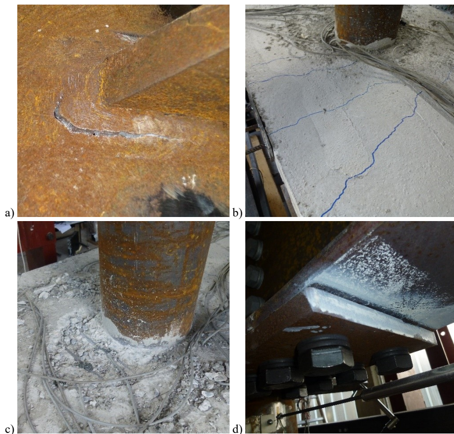
Figure 9.24 Failure modes exhibited in the monotonic test of the two-way C4 specimen: a) cracks in the tensioned welds, b) cracking of the concrete slab in tension, c) crushing of the concrete slab in the contact area, and d) sliding of the external bolted joints
