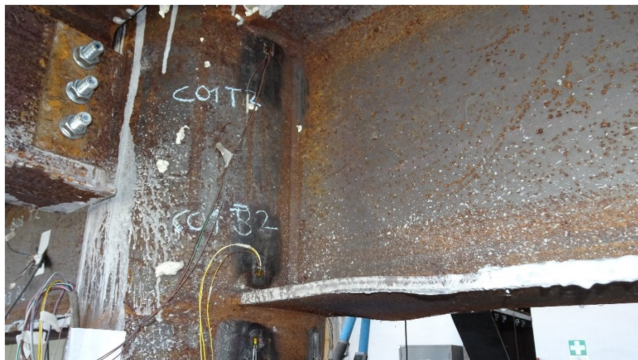
Figure 8.18 Local buckling of the lower compressed flange of the passing-through beam in the main direction of specimen C6
