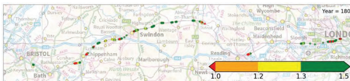
Figure 2: Earthworks vulnerabilities along the London – Bristol railway line in terms of ultimate limit state Factor of Safety
