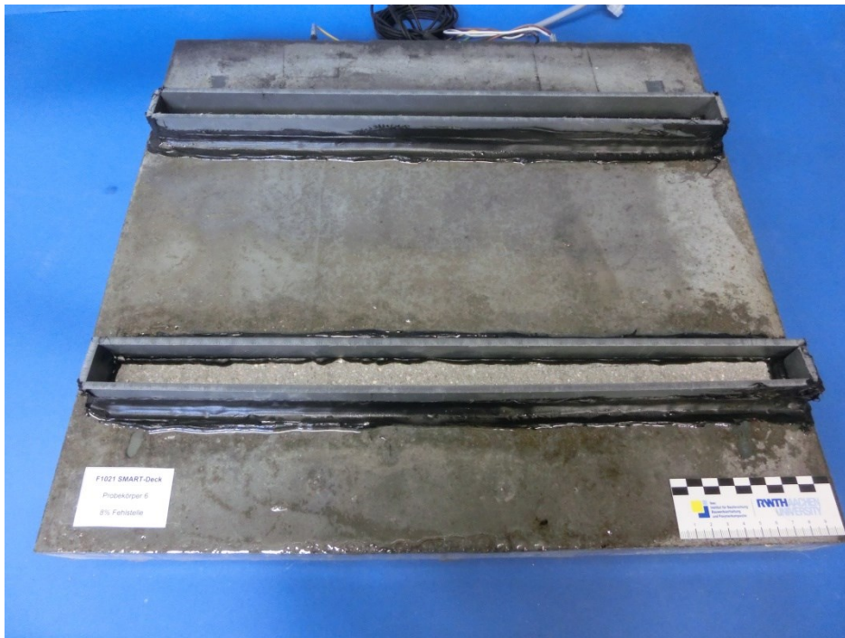
Figure 4.9. Specimen for the detectability-test with two artificial leakages
