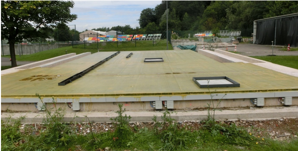
Figure 4.13. Sealed demonstrator with artificial leakages
