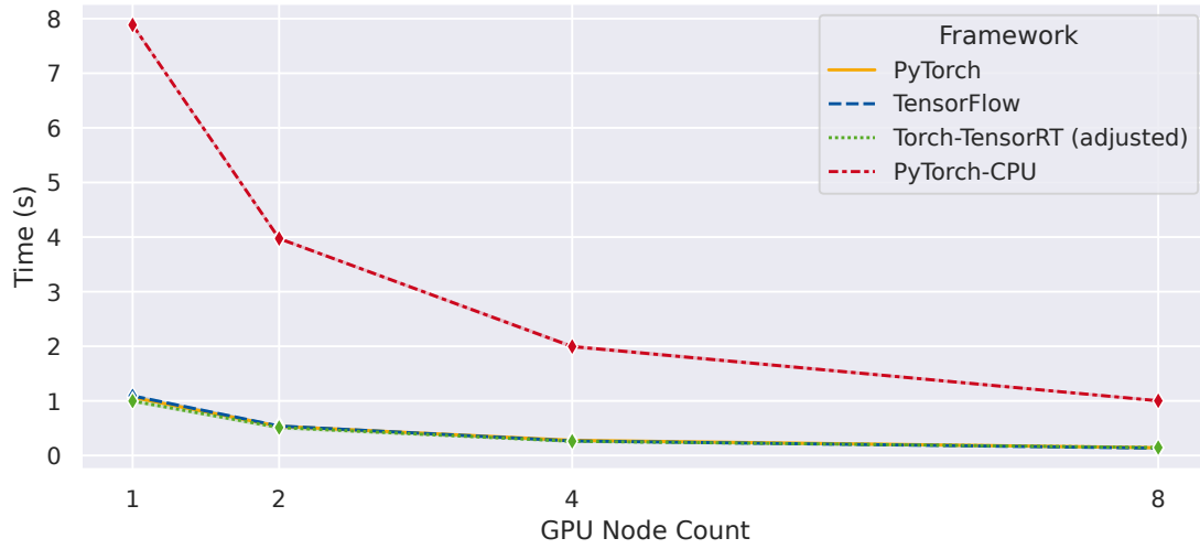
(a) Linear relation between run time and amount of workgroups. The CPU version is much slower than the GPU-accelerated versions.
