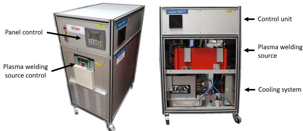
Figure 4.2 – SuperMIG equipment and its structure.
