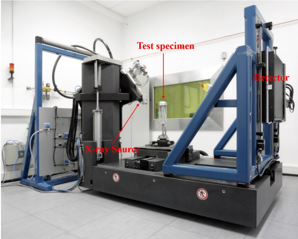
Fig. 3-7. Open X-ray computed tomography system at ZEA-1
