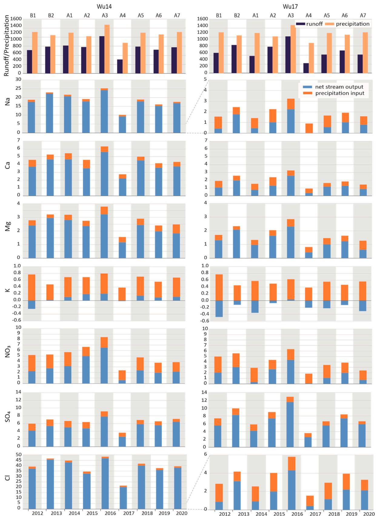
Figure 8. Annual solute fluxes ( \text{t km}^{-2} \text{a}^{-1} ) in stream water and precipitation together with runoff (mm) and precipitation (mm) in the partially deforested Wüstebach catchment (Wu14) and the control catchment (Wu17).
