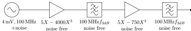
Figure 6.9: System used to compare the system-level noise simulation to a conventional noise analysis.
