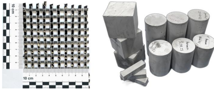
Figure 1 The unimpregnated carbon reinforcement on the left and concrete specimens set on the right
