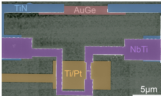
Figure 2.1 – False-colored SEM micrograph of an exemplary extrinsically shunted nanowire Josephson junction on a so-called Shapiro chip . The 10 nm thick AuGe shunt resistor acts as a quasiparticle and noise filter and transforms the sudden and stochastic switching event into the voltage state. The contacts to the nanowire are realized by means of 80 nm NbTi. For the electrostatic tuning, a large bottom gate pad covered with \text{Si}_3\text{N}_4 is used.
