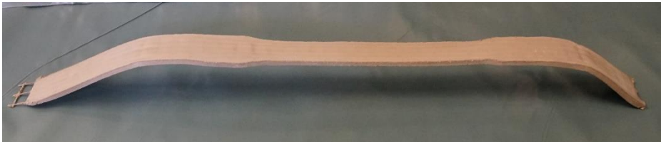
Figure 9 Longitudinal shaping of an ExTRC reinforced with Textile 3.
