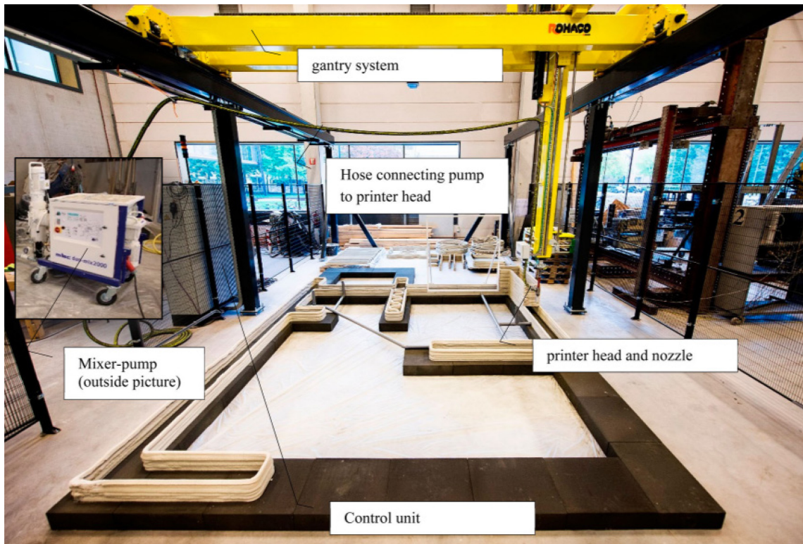
Fig. 2 Printing process using a gantry printer system. Ref.[4]
