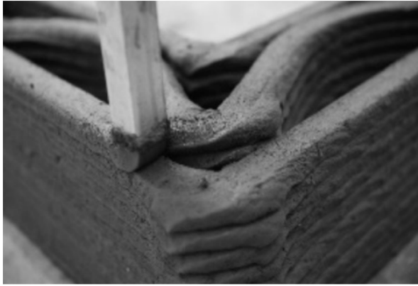
Fig. 14 Excess material deposition while forming a corner. Ref. [24]
