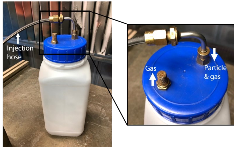
Figure 26: Measuring principle of the PMFR of the powder feeder supplied to the process
