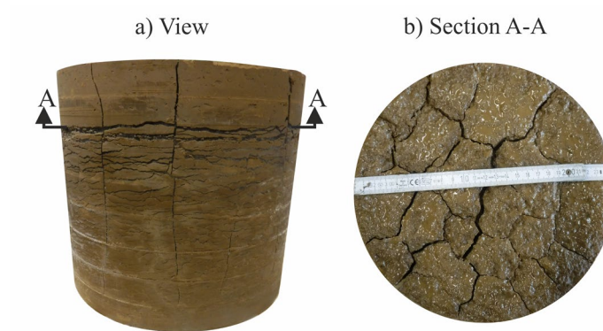
Fig. 6 Longitudinal crack formation of a BF sample
