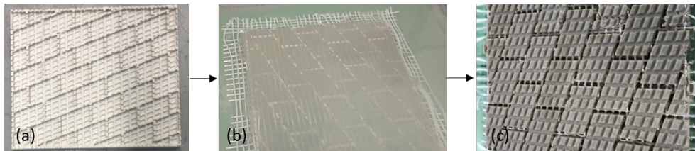
Figure 5.3: Production process of the texture layer: (a) silicone mold, (b) filling the mold and placing textile, and (c) releasing texture layer from mold.
