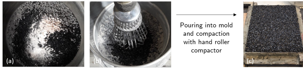
Figure 5.2: Production process of the absorption layer: (a) aggregates, (b) mixing tool, and (c) compacted mixture in mold.
