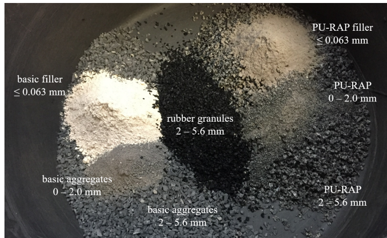
Figure 3.2: PU-RAP and basic material in visual comparison.
