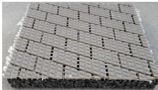
Figure 5.4: Combination of texture and absorption layer.
