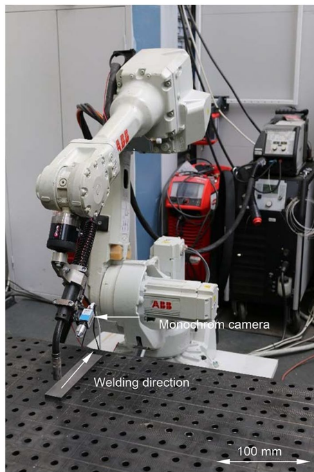
Fig. 6 Experimental set-up for welding tests
