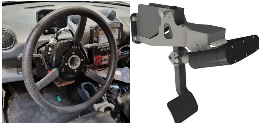
Figure 10. Selected steering wheel actuators and pedals for dynamic vehicle control.
