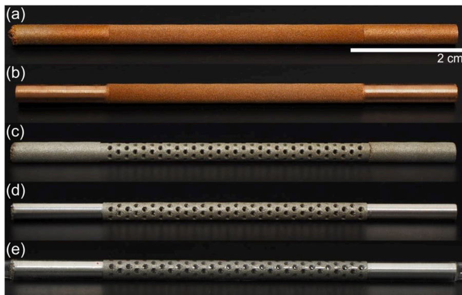
Fig. 3. Processing steps involved in cathode and anode production. (a) 3D printed cathode after removal of residual copper powder and (b) after polishing the solid ends to a smooth finish. (c) 3D printed anode after removal of residual stainless steel powder, (d) after turning the ends on a lathe and (e) after shrinking a commercial Nafion™ tubing, thereby creating a MEA.
