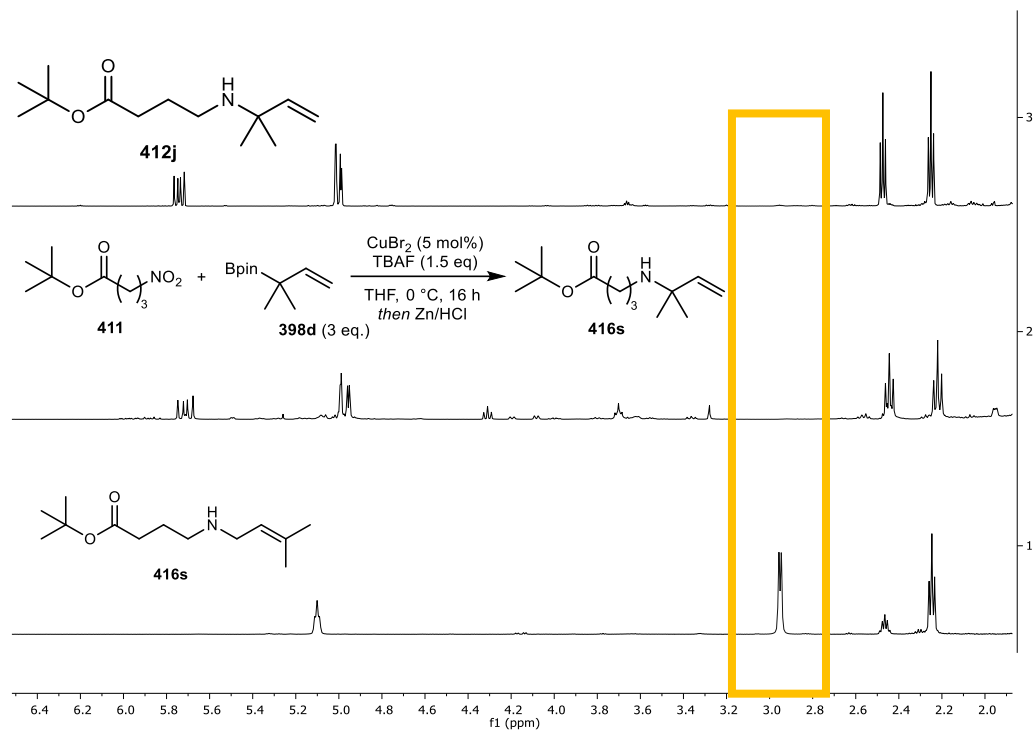
Figure 14. Determination of the regioselectivity of the reaction with nitro compound 411 and prenylboronate 398d via ^1\text{H} -NMR.
