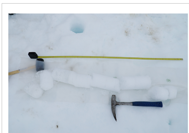
FIGURE 4 Ice core collected at the dome of Collins glacier by the Planetary Sciences & Remote Sensing group at Freie Universität Berlin at the beginning of 2024.
