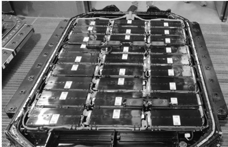
(a) Audi E-Tron 50 71 KWh battery during teardown, with 60 Ah Samsung SDI prismatic cells 142,143
