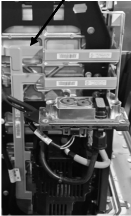
Plastic carrier with many short bus bars
