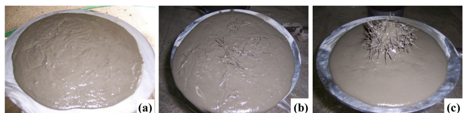
Fig. 3 Dispersibility of fibres within FRC: a Grade 1, b Grade 2, and c Grade 3
