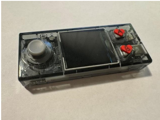
Figure 5: CyberPi controls the secondary robots
