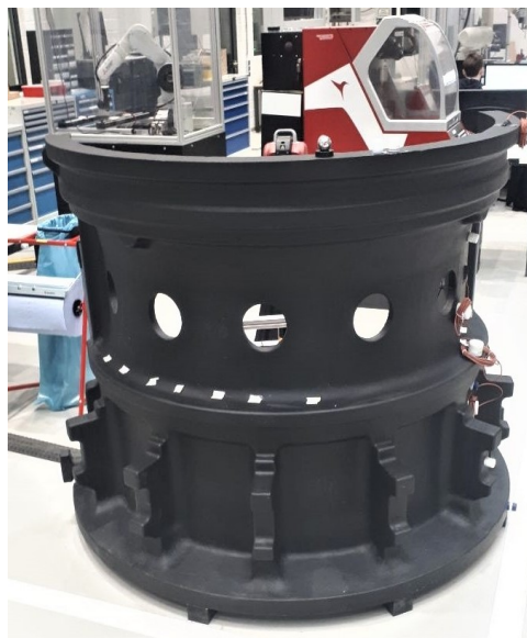
Figure G.2: Task poses indicated by stickers for marking on the turbine.
