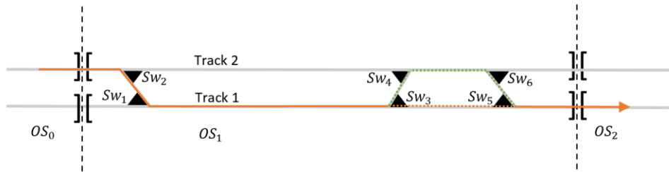
Figure 14: Train routes along different sets of switches
