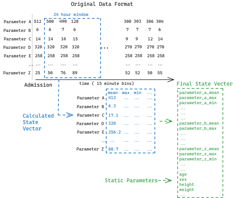
Figure 4.2: Visualizes the data structure for model training. Past data for all parameters is described through different statistics. The resulting matrix is transformed to a vector and the static parameters are appended. This vector is then used with the XGBoost predictor.
