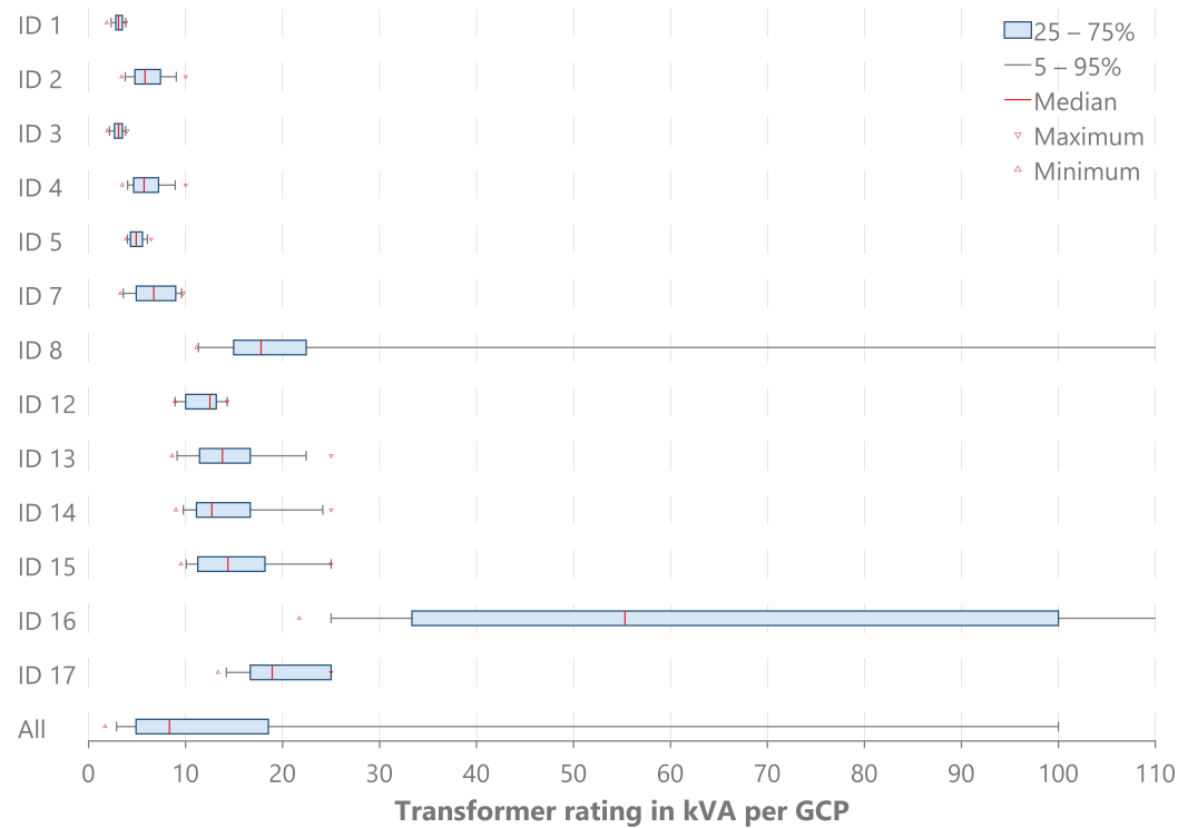
Figure A3. Statistical evaluation of the transformer rating per GCP in the different meta-clusters in kVA.
